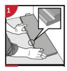
Note: This spacing must also be maintained between the floor and all vertical surfaces, including cabinets, posts, partitions, door jambs, door tracks, fireplaces, etc...
